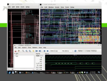
Fedora's HDL simulation environment enables you to verify the functional and timing models of your design.
