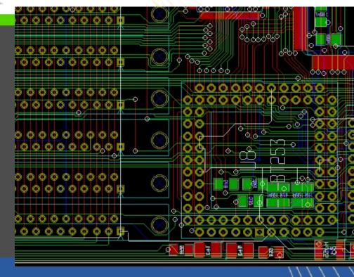
Includes a rats nest feature, design rule checking, and can provide industry standard RS-274-X (Gerber), NC drill, and centroid data (X-Y data) output for use in the board fabrication and assembly process.
